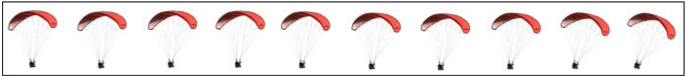
In slow flight, during a sudden stop of the action on the brakes → the glider stalls and take speed
