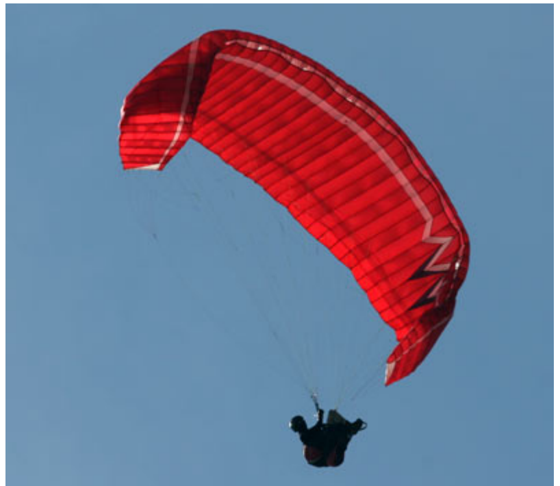
Photo 4-18: Big ears. This maneuver is especially suitable well for crossing a turbulent zone.
