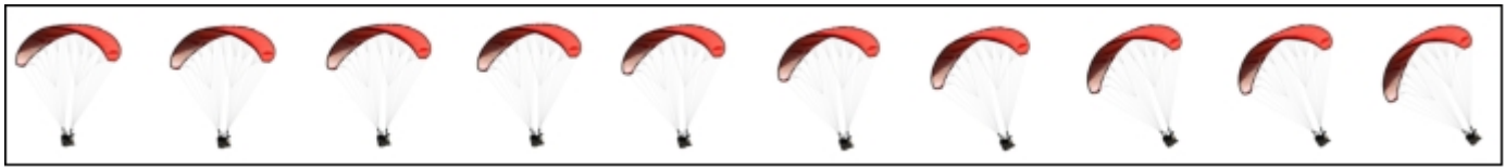
Figure 4-8: Forward pendulum movement of the pilot when using the brakes after a quick or accelerated flight. Caution: In an extreme case, the angle of attack can increase so much that the air flow picks up dynamic stall. Canopy swing during a sudden stop on brake action (e.g., after stall). Caution: In an extreme case, the glider is powered on the upper surface for a moment and closes along the leading edge.
