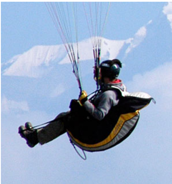
Figure1-4: Extended position in the harness. This position delays the rotation of the pilot around the vertical axis: attention during a quick turn!
