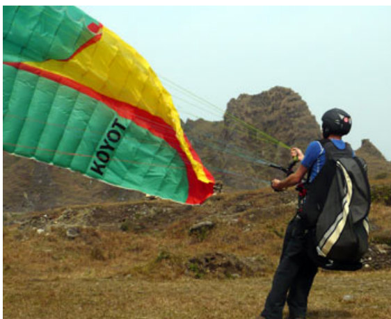
Inflation front wing with the method of crossing the arms.
